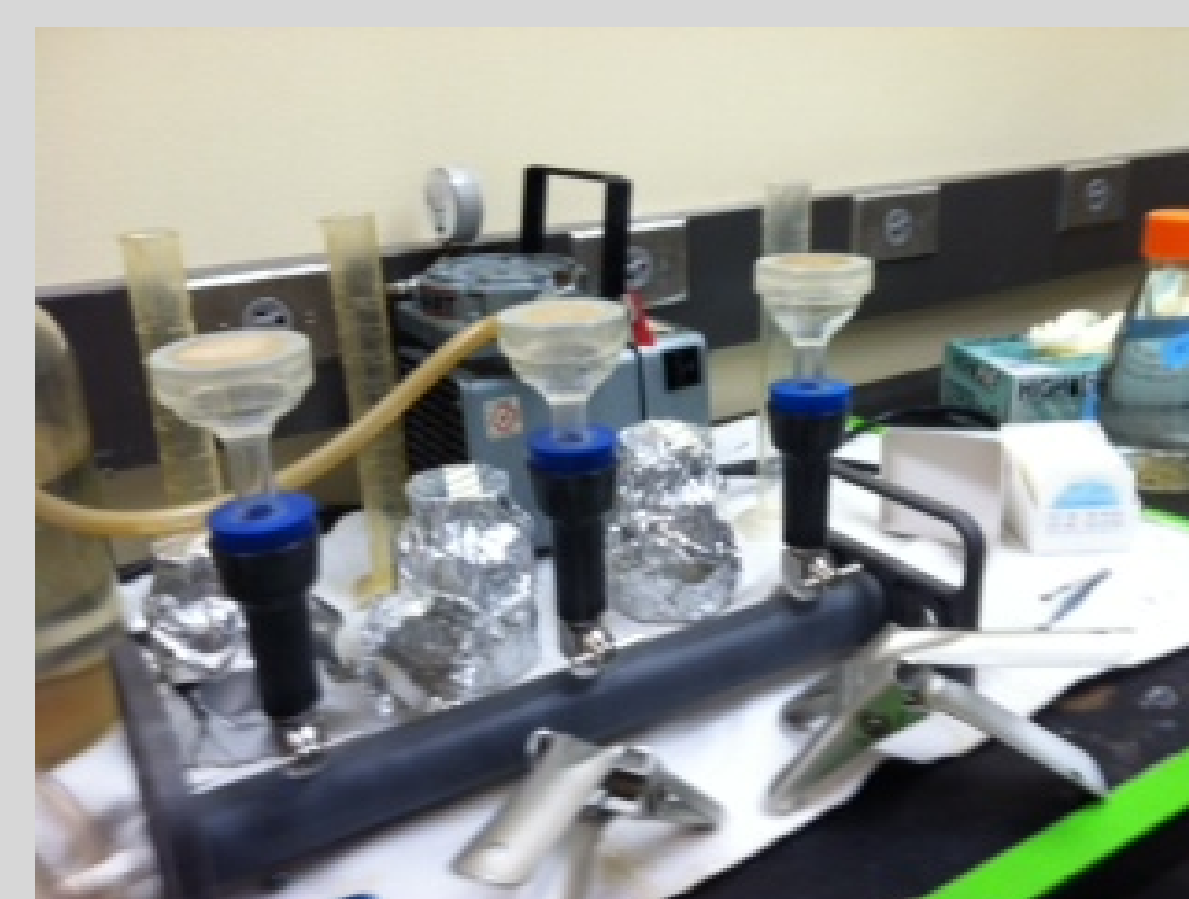
Vacuum filter set-up.
