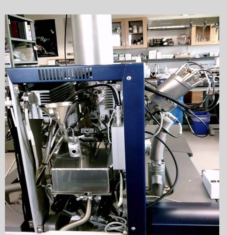
TOF.SIMS*5 uses liquid nitrogen and pictures to evaluate the amount of Elements and compounds
