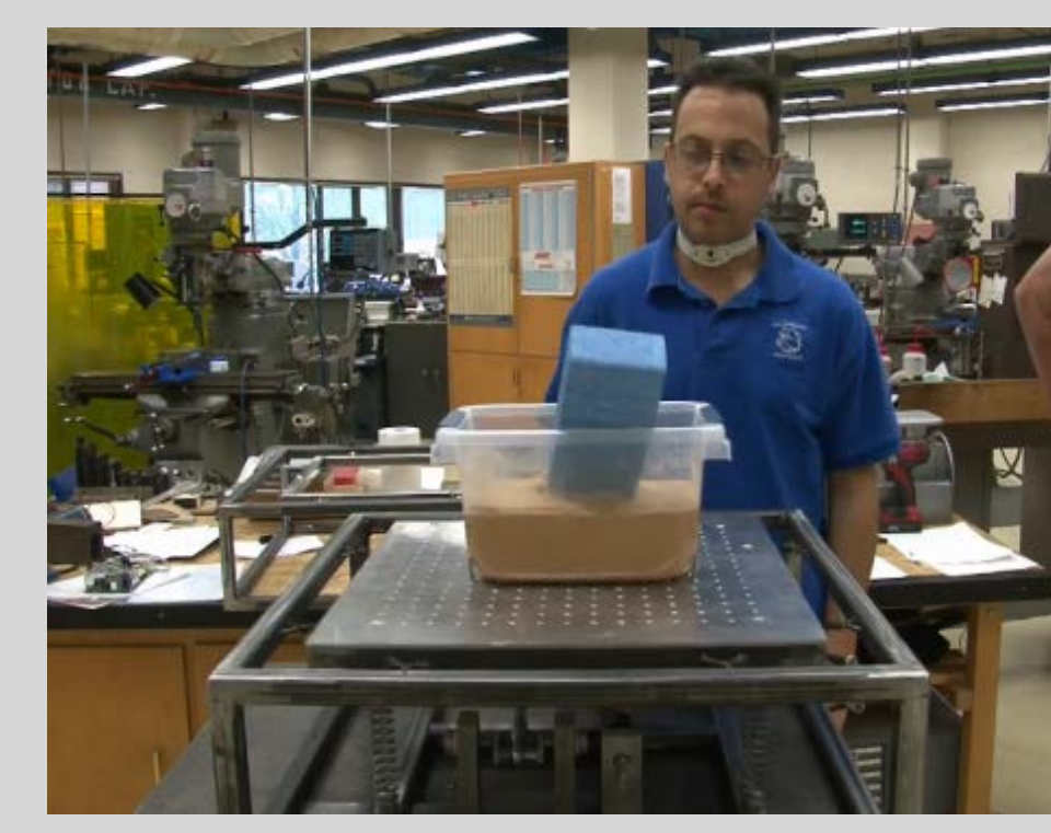
Shaker table trial with saturated sand
