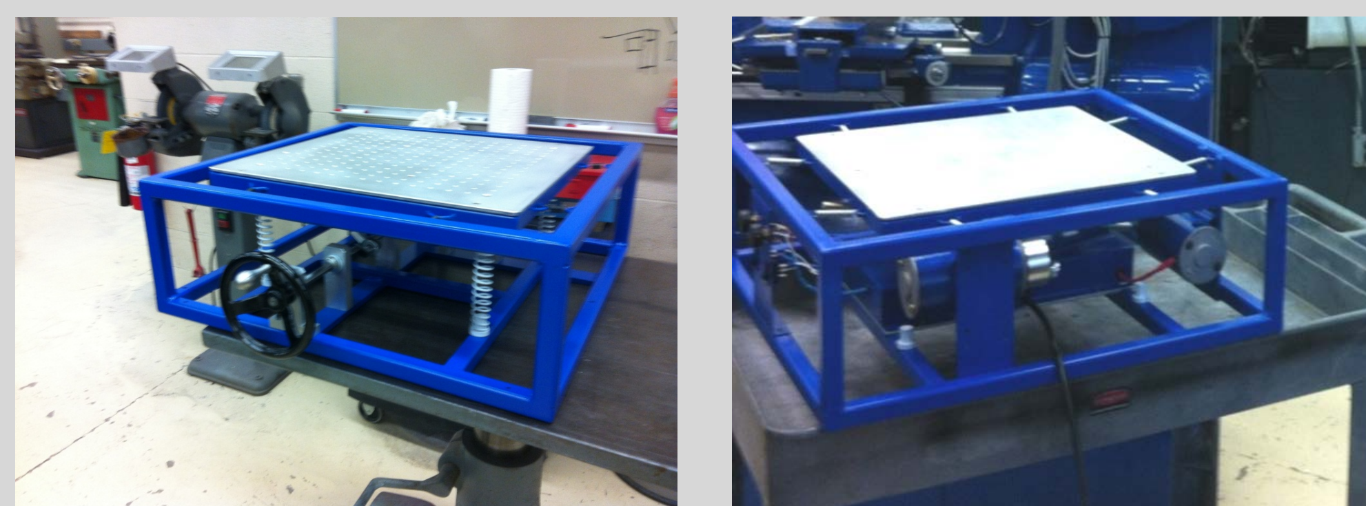
Completed shaker tables: crankshaft and motorized designs
